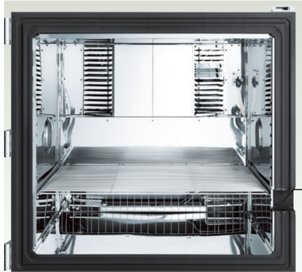
Inside of the ARS-1100-5 chamber
