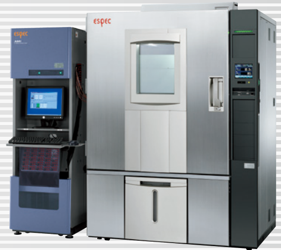
Example of AMI Connected with a temp. & humid. Chamber
